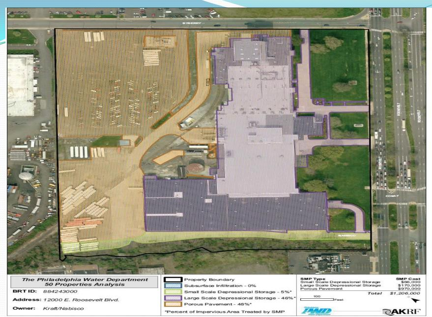
Approximately 71% impervious (total area 1,203,581 sf). Large and small scale depressional storage and porous paving.
